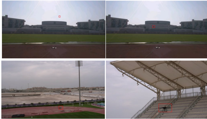
Fig. 4. Visualization of drone surveillance system in field test. The drones are captured by a still camera on the ground (first row) or a camera mounted on a flying drone (second row)
