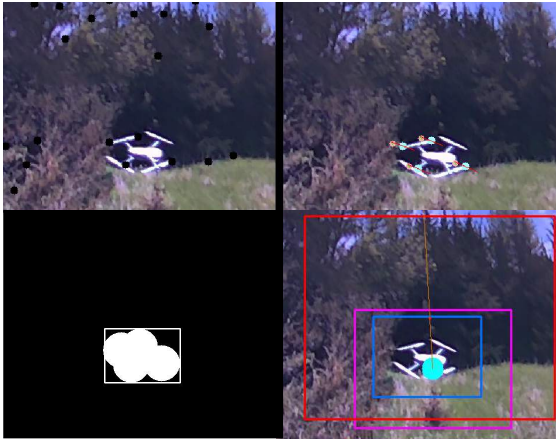
Fig. 5. Estimated image features on tracked UAV
