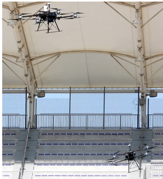
Fig. 1. Tracker and pursuer UAV with mounted PTZ Camera
