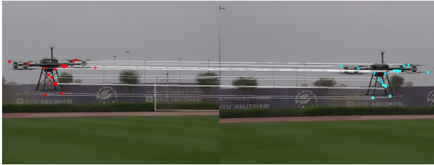
Fig. 4. Image feature matching between successive frames
