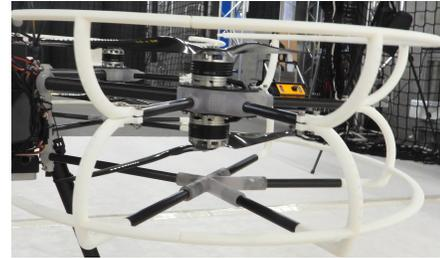
Fig. 3: Protective propeller bumper structure
