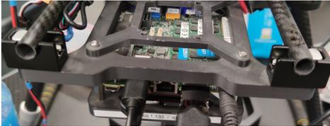
Fig. 2: Intel NUC mounting assembly
