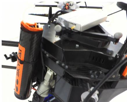
Fig. 6: Parachute and Video Transmitter
