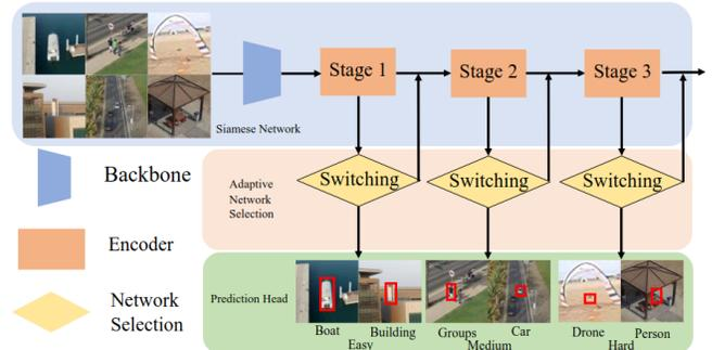
Fig. 1: Overview of the proposed tracking strategy for adaptive inference based on the input scenarios complexity. In most cases, a shallow network with only one encoder block is sufficient to track objects. An array of encoder blocks with increasing representative ability are employed to deal with more challenging cases. The optimal computational graph is determined by the network selection module.
