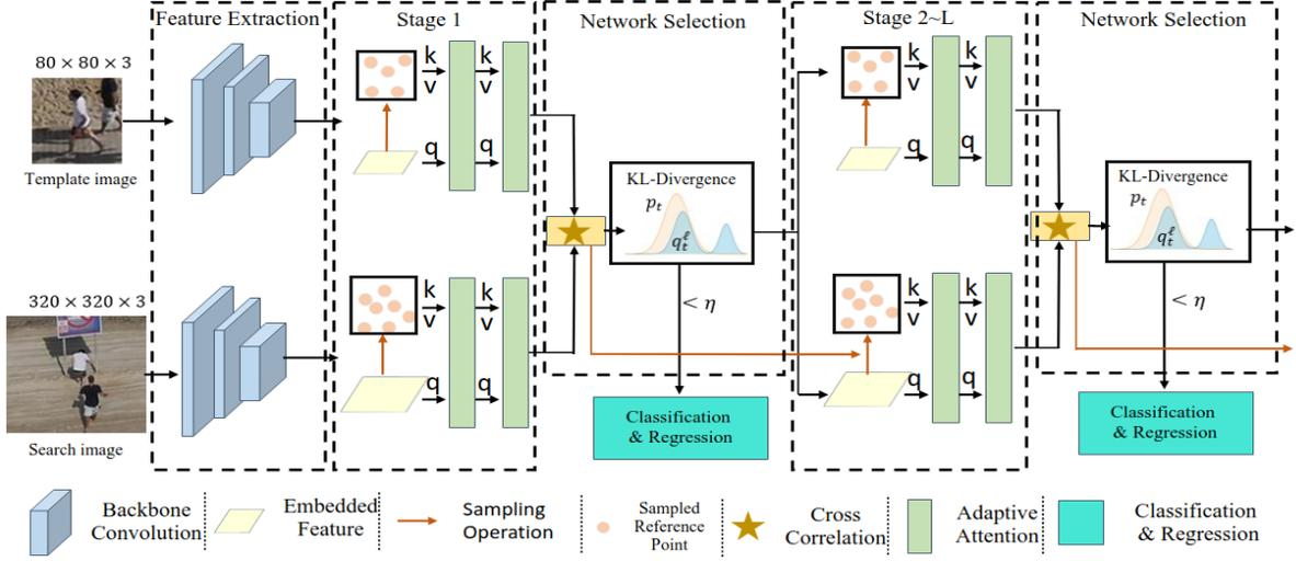
Fig. 2: The overview of the SiamATN tracking framework. It consists of a shared backbone followed by encoding stages and corresponding prediction head. The optimal exit depth is determined by Network Selection module. Auxiliary stages will be activated if the KL-divergence is over  $\eta$  and perform self-attention over adaptive selected point set. The procedure will continue until the exit criterion is satisfied or the network reaches depth maximum.
