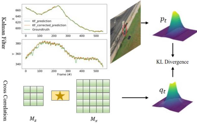
Fig. 3: Visualization of network selection workflow. The trajectory is recorded and predicted by a Kalman filter (KF). The expected distribution  $p_t$  (red circle in the frame) generated from KF prediction is compared with estimated distribution  $q_t$  generated from cross correlation, yielding KL score for network selection. The line plots are X&Y coordinates from KF predictions  $\hat{b}_t^-, \hat{b}_t^+$  and ground truth  $b_t$ .
