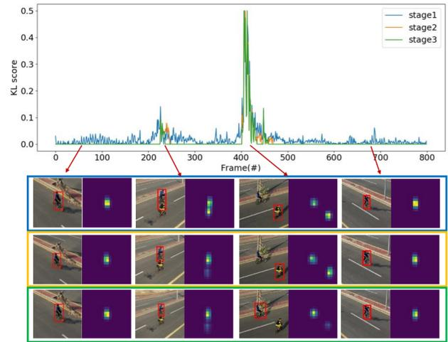
Fig. 5: A long-term tracking example where the tracking network is adaptively selected according to the KL-divergence score. The bounding box and centerness score predictions for each stage are shown in row 2 to row 4.
